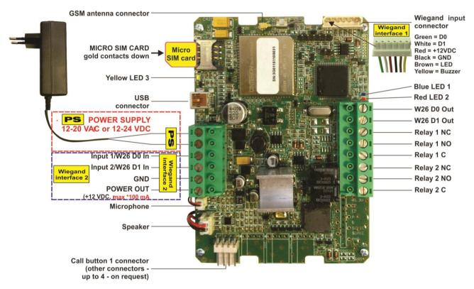
Figure 1: SOLO: Connection diagram
