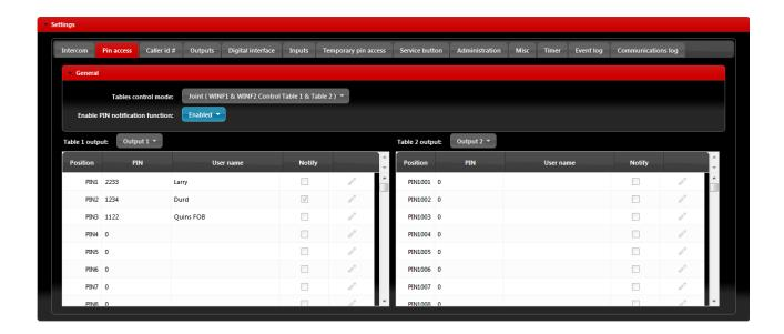
Figure 20: WEB Server-Global enabling of the notification function.
