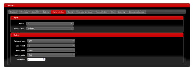
Figure 7: WEB Server-First Wiegand interface support.
