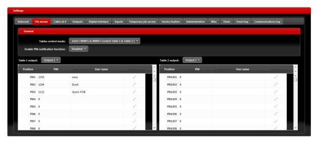
Figure 9: WEB Server-Adding Wiegand devices with permanent use.
